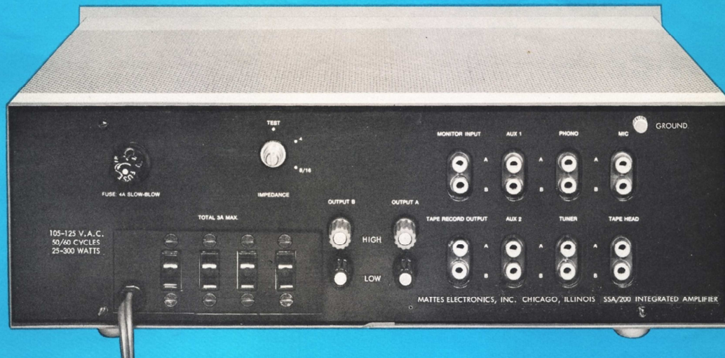
Rear of unit with multiple inputs, output terminals, test/impedance switch and AC outlets for other components.
